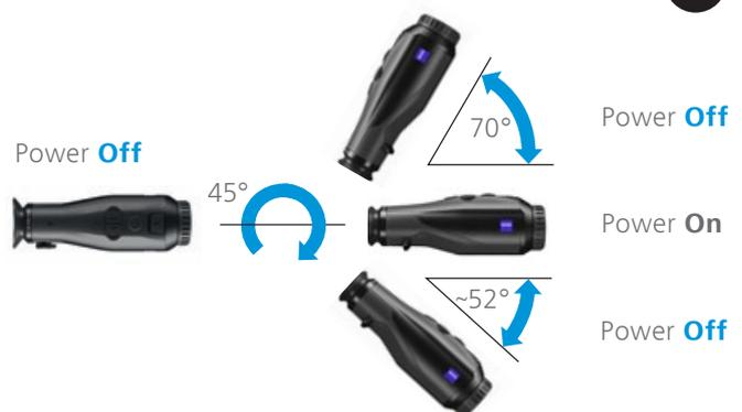
**When Smart Standby is enabled, the device automatically switches to power-saving mode when you tilt it up more than 70° or down more than 52.5°.** If you place your thermal imaging camera on an edge when not in use while up on your raised hide, it automatically switches to intelligent standby mode – at a 45° angle to the left or right.
