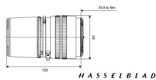
No infrared correction needs to be applied. The lens therefore comes without an infrared-index. The focussing ring can rotate beyond infinity to allow use of this lens in a variety of temperature conditions.
