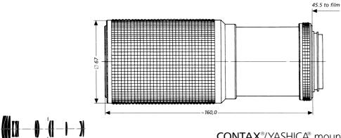
The 80-200 mm Vario-Sonnar® T\* f/4 lens from Carl Zeiss is a light, one-touch zoom lens which provides very good image quality over the entire focal length range. As with the 35-70 mm Vario-**Sonnar**<sup>®</sup> T\* f/3.4 lens, the same ring is used for zooming and focusing.
