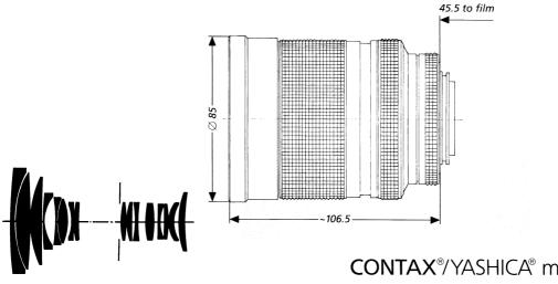
The 35-135 mm Vario-**Sonnar**® T\* f/3.3-4.5 lens from Carl Zeiss is a 3.8x zoom lens. Its superb image quality makes it another valuable addition to the existing range of Carl Zeiss Vario-Sonnar® lenses for the **Contax**<sup>®</sup> SLR Camera System. The image quality is very good even at the shortest focusing distance of 1.2 m. This Vario lens has also been manufactured using
