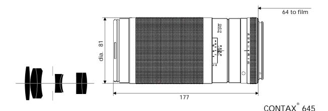
The **Sonnar**<sup>®</sup> T\* 4/210 lens is an autofocus telephoto lens similar to a 135 mm lens on a 35 mm Contax<sup>®</sup> SLR. The optical system was designed using the latest technology, incorporating internal focusing (IF) and the most recent optical glass types. It shows outstanding performance.
